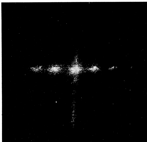
FIGURE 4. Optical diffraction pattern from transmission of 6328 Å light through a crystal of (\text{CH}_3\text{NH}_3)_2\text{MnCl}_4 at room temperature.
